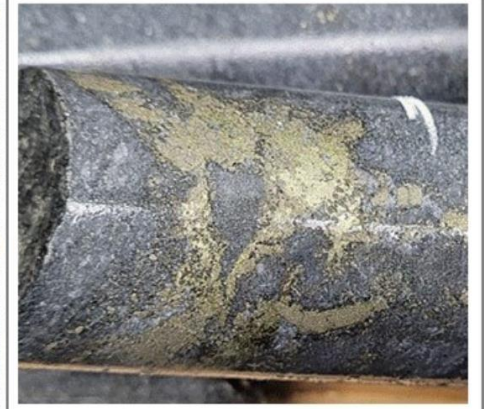
WC-21-188: 148-149m with 1.0m of 1.35 g/t Au; patchy replacement texture pyrite and chalcopyrite in greywacke host
