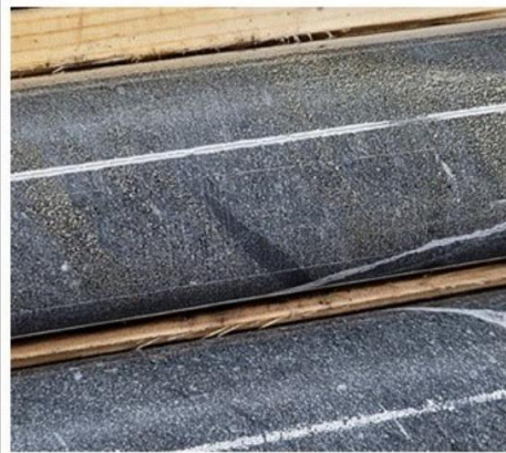
WC-21-188: 119-120m with 1.0 m at 4.69 g/t Au; disseminated finely bedded pyrite in mostly greywacke host; note black argillite clast
