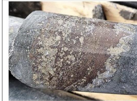
WC-21-182: 83-84m with 1.0m at 1.04 g/t Au; bedded sphalerite core with pyrite dominant margins define sulfide (clast?) in sediments; weakly re-mobilized sulfides in adjacent white quartz veining
