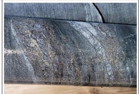
WC-21-186: 126-127m with 1.0m at 3.5 g/t Au; mixed pyrite, pyrrhotite and sphalerite in mildly sheared bedded sulfides with late quartz veinlets
