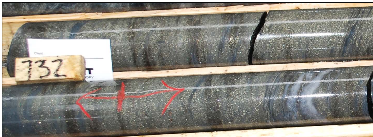
FIGURE 7.23 BUCKSHOT PYRITE IN WEST DEEP ZONE DRILL HOLE TPW-10-30
