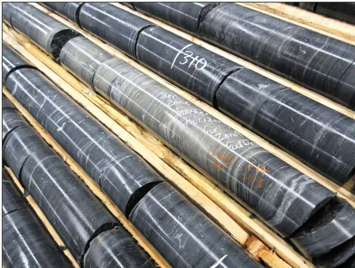
FIGURE 7.16 SERICITE ZONE MARKER HORIZON IN ZONE #9
