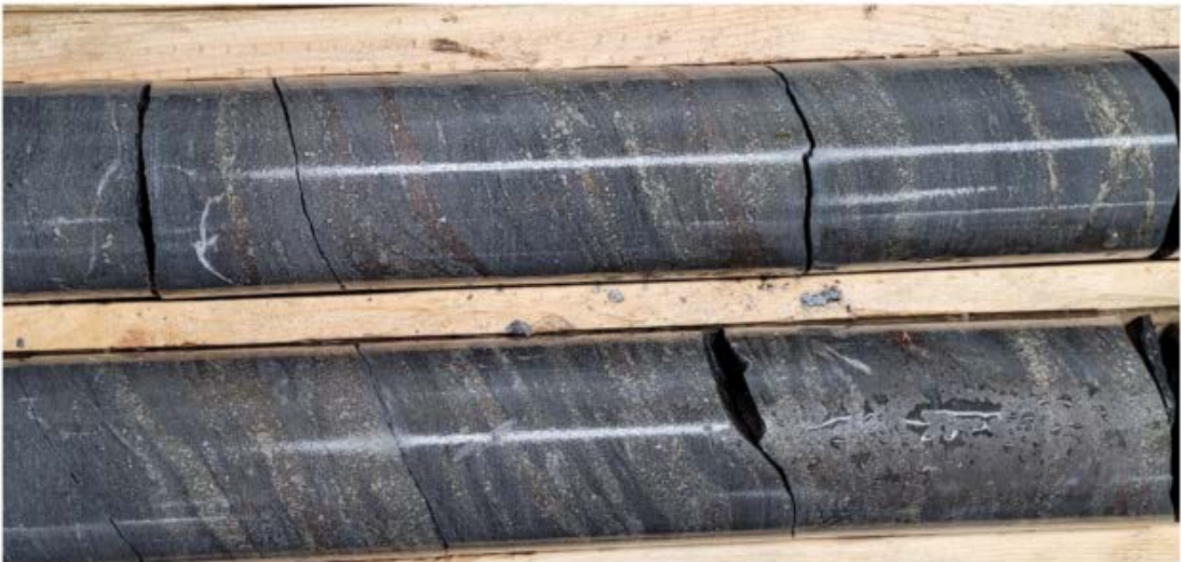
FIGURE 3: WC-21-172 Core 9.98 g/t over 1.0 m (233 – 234 m)
