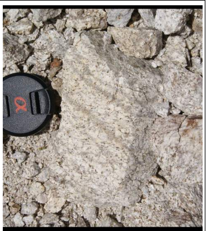
Figure 7-6 Pegmatitic Textured Phase of Granodiorite: note banded quartz – k-spar(?) veining and minor white mica alteration of feldspars
