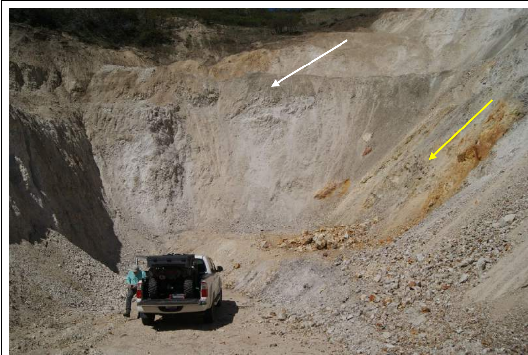
Figure 6-3 Mineral Point, LLC Bulk Sampling Open Cut Pit at Neal (2015-2016)- Author completing open cut examination on April 27, 2019; vein remnants with notable silicification, quartz veining and iron oxide after pyrite (red-brown material) on right (yellow arrow); hangingwall fault zone with associated clay – white mica alteration (white arrows)
