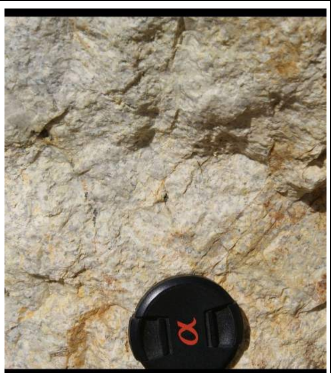
Figure 7-11b Hard Flinty White Silicification- main vein strong silicification of granodiorite protolith
