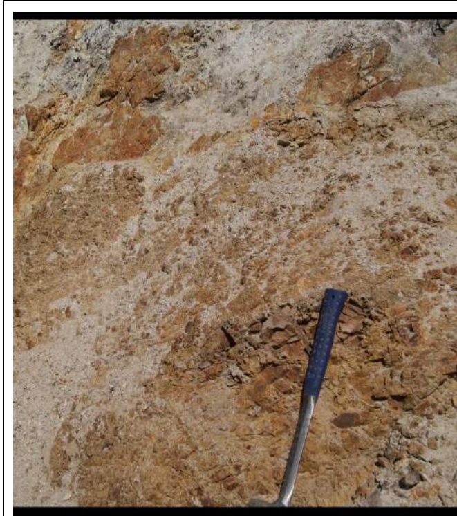
Figure 7-5 Lamprophyre Dike: partially altered in main vein zone of open cut; macroscopically, the dike appears to be pyroxene dominant
